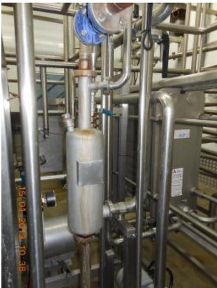
**Figure 9. Milk pasteuriser with steam injection**
