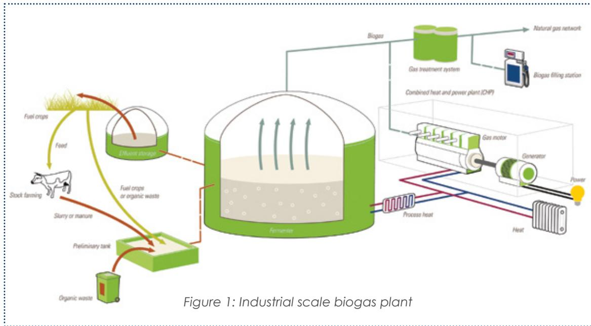
Figure 1: Industrial scale biogas plant
