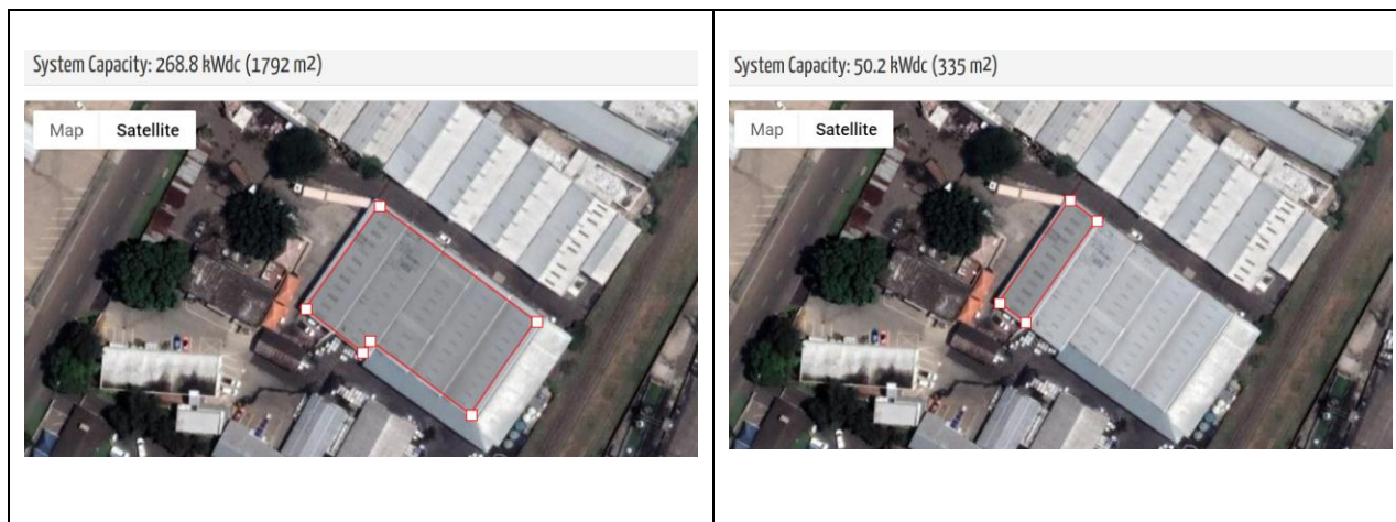
Figure 1: The roof view of Aquatrade with low and high Solar System Installation capacity.
