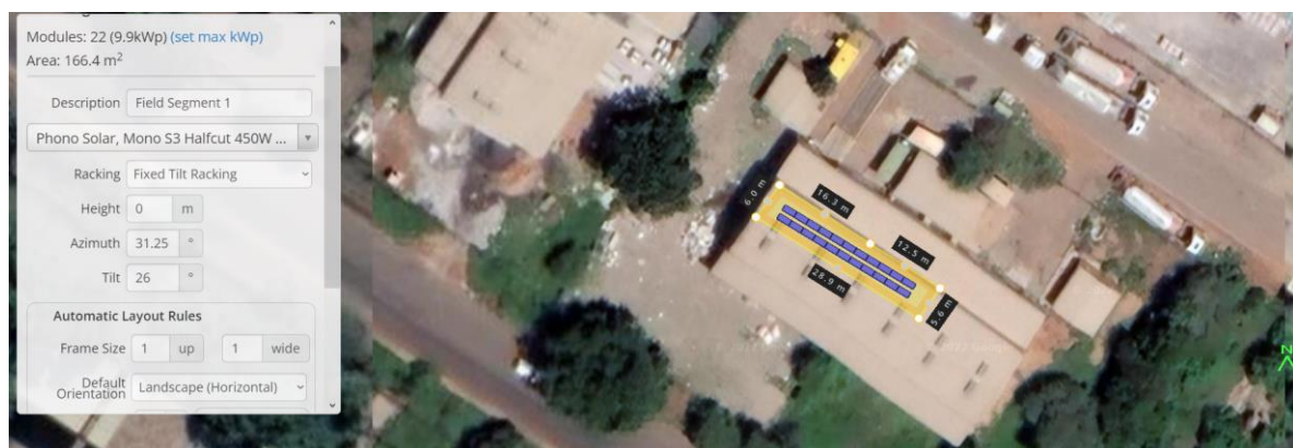
Figure 4: The roof space of Ecocare and its maximum as well as the maximum solar system installation capacity
