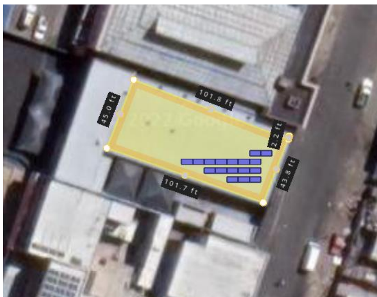
Figure 7 HelioScope Rooftop PV System Design
