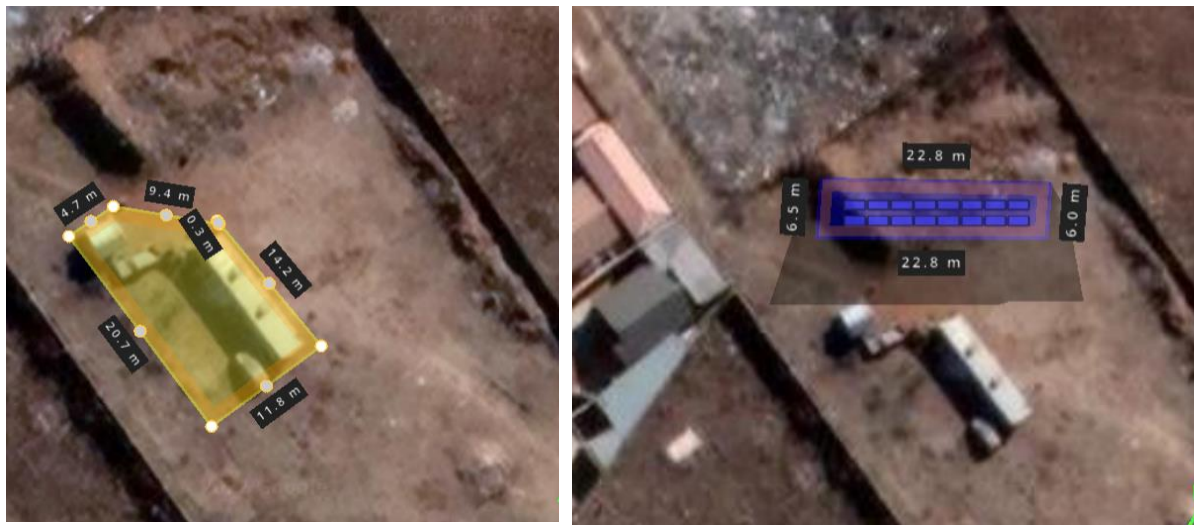
Figure 5. The roof space of Mr Bin Cleaner and Waste Management and its maximum as well as the maximum solar system installation capacity
